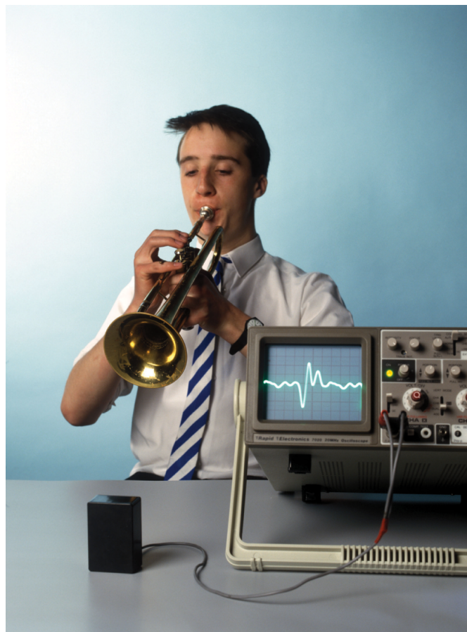
Image P12.04 To display the vibrations of a musical note, it is converted to an electrical signal by a microphone and displayed on the screen of an oscilloscope. The trace on the screen shows the regular pattern of vibration of the sounds.
