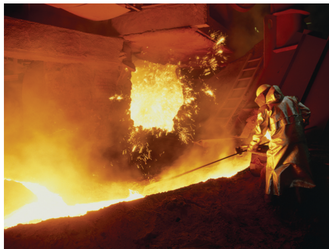
Image C9.01 A worker in protective clothing takes a sample from a blast furnace in a steel works.
