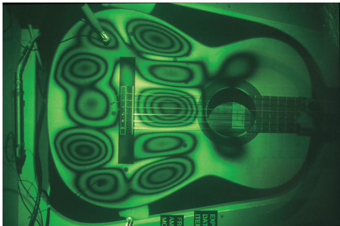
Image P12.01 Although the player only touches the strings of a guitar, the instrument's whole body vibrates to produce the notes we hear. This is shown up in this image, produced by shining laser light onto the guitar. Different notes produce different patterns of vibration, and this helps to give each note its particular quality.
